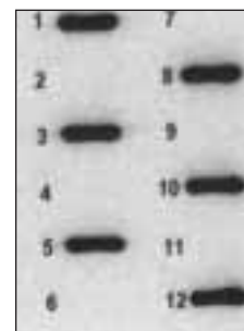
Figure 1 Slot-blot analysis showed no detectable sample-to-sample contamination within or between extraction runs. The single-use reagent cartridges, filter barrier pipet tips, and the linear extraction process all contribute to decreasing the possibilities of cross contamination during DNA purification.
