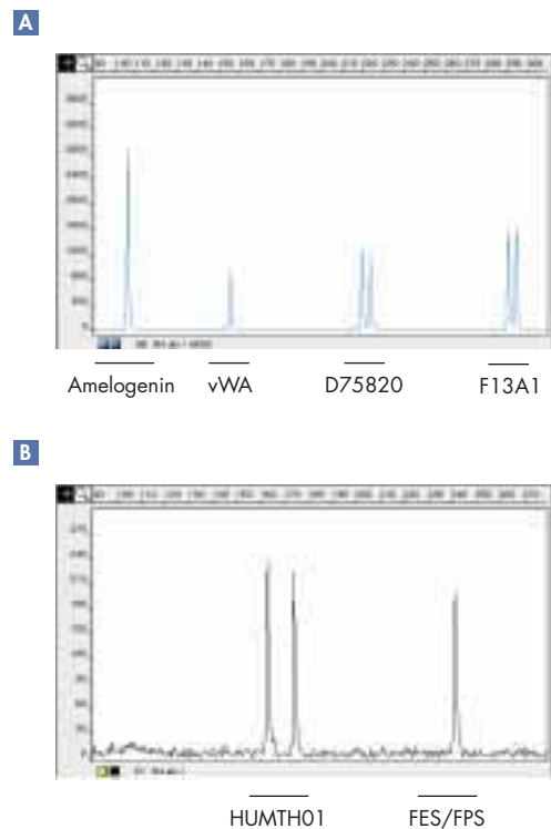
Figure 2 The indicated STR loci were analyzed by multiplex PCR using fluorescently labeled primers. Fluorescent peak traces were obtained using the A FAM or B HEX channel of a DNA sequencer.
