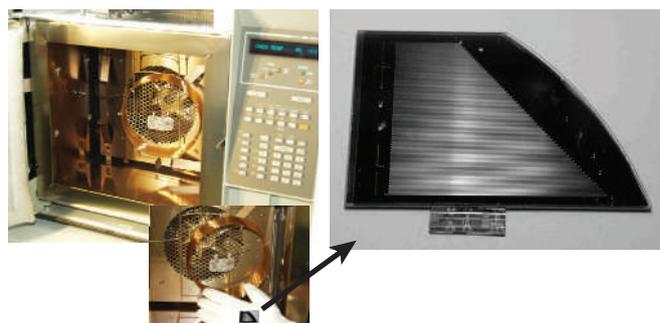
**Figure 1** Examples of the miniaturization of separation techniques. The figure compares the size of a commercial gas chromatograph and column with that of a microscaled column on a chip. (Photo of microscaled column courtesy of J. Müller, Institut für Mikrosystemtechnik, Technische Universität Hamburg-Harburg, Germany.)
