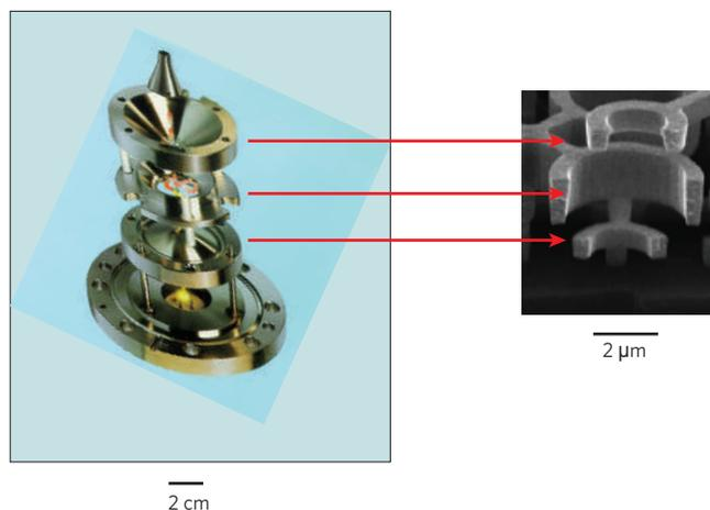
**Figure 4 | Ion traps as an example of miniaturization in detection.** The left panel shows the ITD700/800, a conventional ion-trap detector (image courtesy of Thermo Electron, Bremen, Germany); the right panel shows a scanning electron micrograph. The arrows indicate the two end caps and the ring electrode. Reprinted, with permission, from ref. 62.
