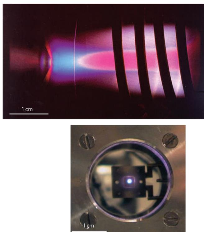
**Figure 2 | Plasma detectors, an example of miniaturization in detection.** Photographs of an inductively coupled plasma with power consumption of 1 kW and a microhollow cathode plasma of less than 1 W. The whole of the microhollow cathode has a diameter of 100  $\mu\text{m}$ .
