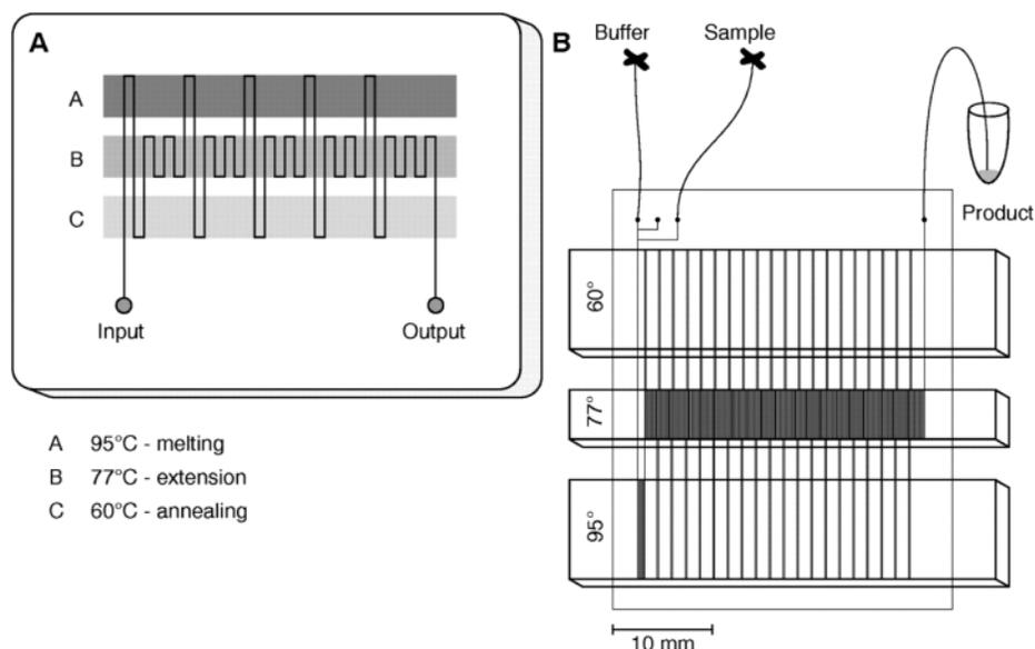
**Fig. 3** Continuous-flow PCR on a chip: (A) schematic of chip layout; (B) schematic of experimental set-up. Reprinted with permission from *Science* (Washington, D. C.), 1998, **280**, 1046. Copyright 1998 American Association for the Advancement of Science.
