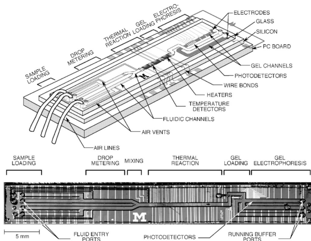
**Fig. 6** Schematic of an integrated nanolitre DNA microdevice incorporating fluidic channels, heaters, temperature sensors and detectors. Reprinted with permission from *Science (Washington, D. C.)*, 1998, **282**, 484. Copyright 1998 American Association for the Advancement of Science.
